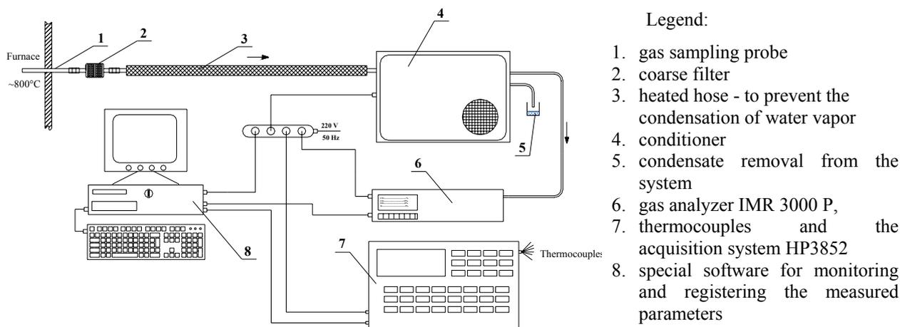
**Figure 3: Scheme of the gas analysis and temperature acquisition system**
