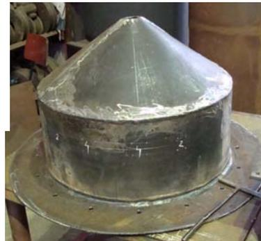
Figure 12. Lower flange / FB bottom under construction
