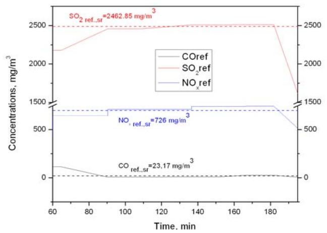
**Figure 6. Regime I – concentrations of CO, SO<sub>2</sub> and NO<sub>x</sub> at reference O<sub>2</sub> content (O<sub>2,ref</sub>=7%)**
