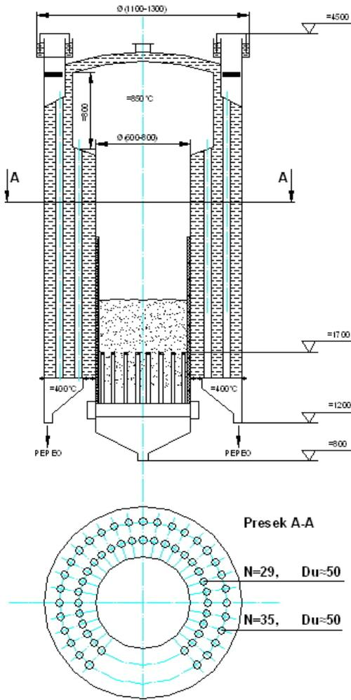
Figure 11. Schematic of industrial FB demo-boiler
