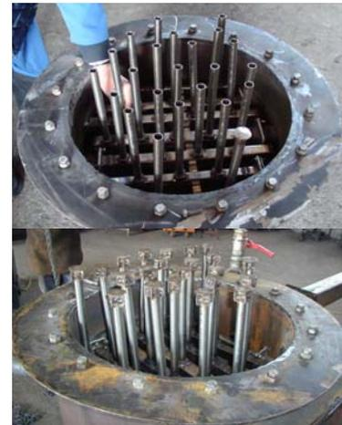
Figure 13. Installation of bubble caps for fluidization onto the fluidization air distributor
