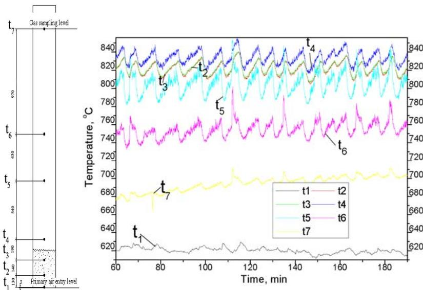
**Figure 7. Regime II – temperatures within the furnace (measured values), placement of the thermocouples in the fluidized bed furnace - on the left**
