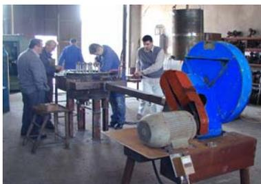
Figure 14. Mounting of the fluidization fan onto the fluidization air/gas distributor
