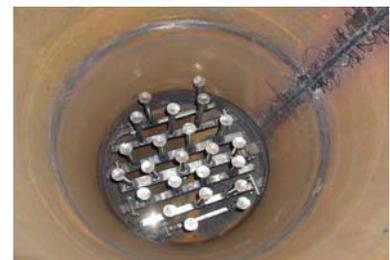
Figure 16. Distributor appearance, observed from the top of the furnace
