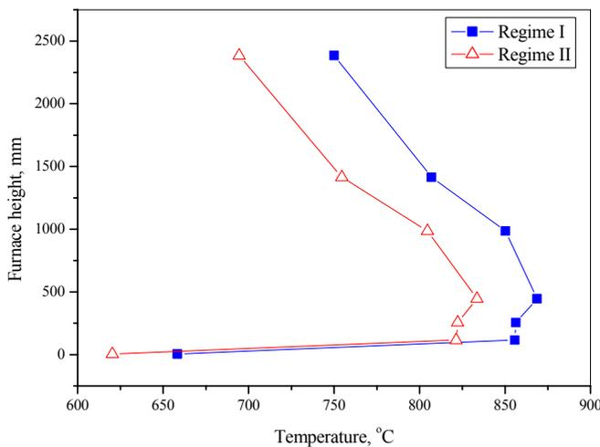
Comparison of average temperature profiles along furnace height, showed in Figure 10, enables comparison of the regimes. Temperature profiles are very much alike, because of the control method used, as well as due to the design characteristics of the furnace itself.
