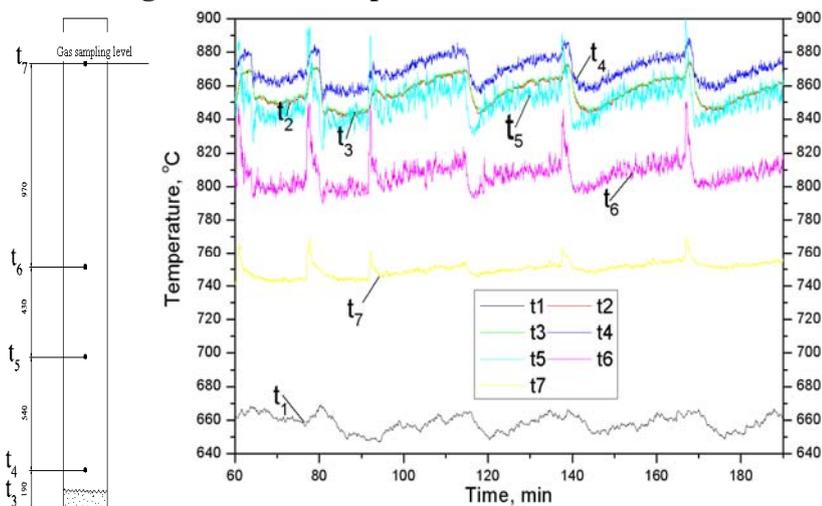
**Figure 4. Regime I – temperatures within the furnace (measured values), placement of the thermocouples in the fluidized bed furnace - on the left**
