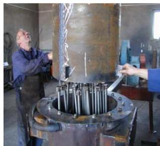
Figure 15. Installation of the furnace shell onto the air distributor
