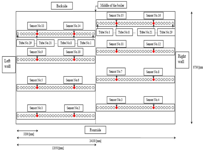
**Figure 4: Positioning of the weight sensors over the cross-section.**
