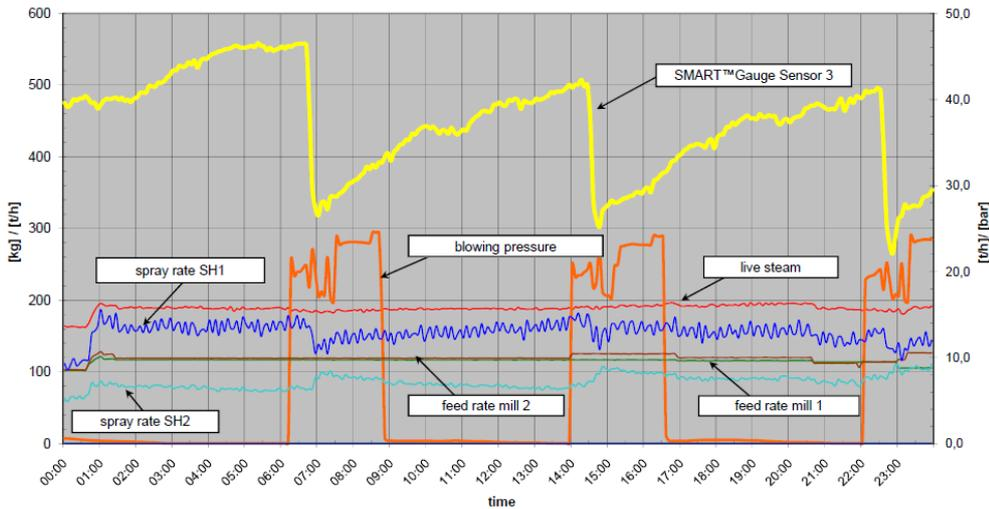
**Figure 1: Signal response of weight measurement at a superheater.**
