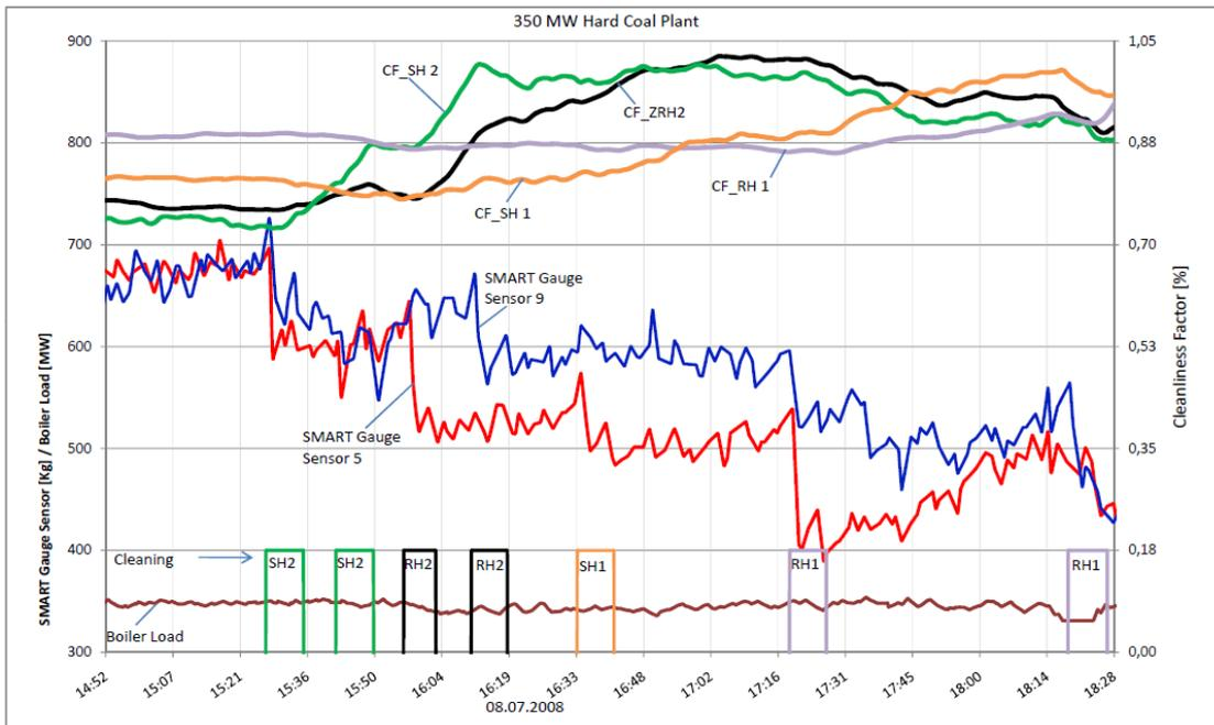
**Figure 5: Typical signal response of weight development, Cleanliness Factors and boiler cleaning actions.**
