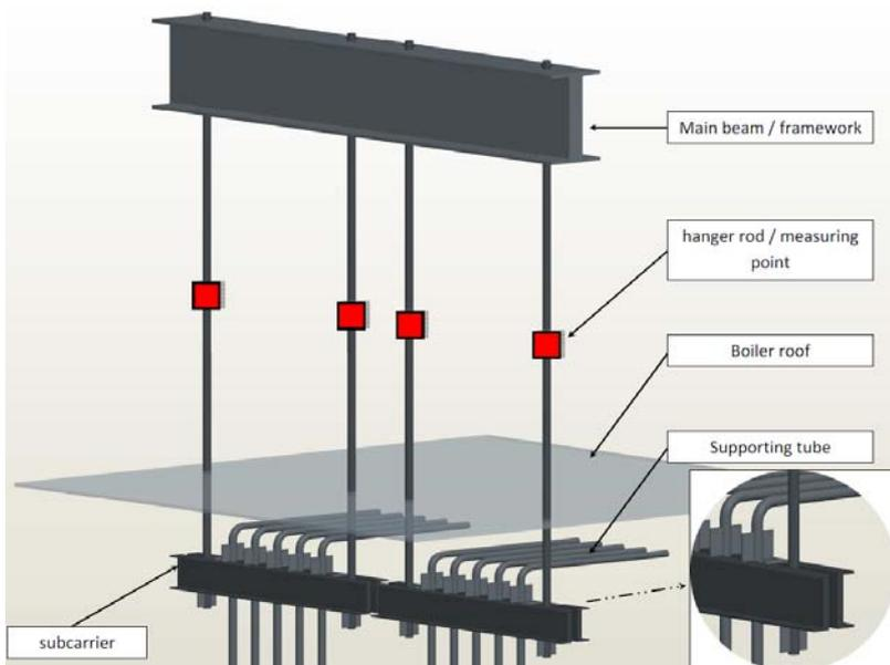
**Figure 2: Suspension of heat exchanger bundles with mounted weight sensors.**
