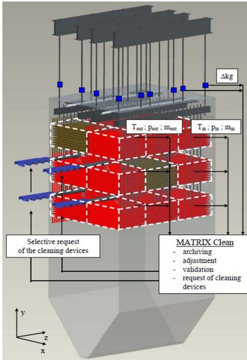
**Figure 3: Split of the superheater area in zones for selective deposit analysis.**
